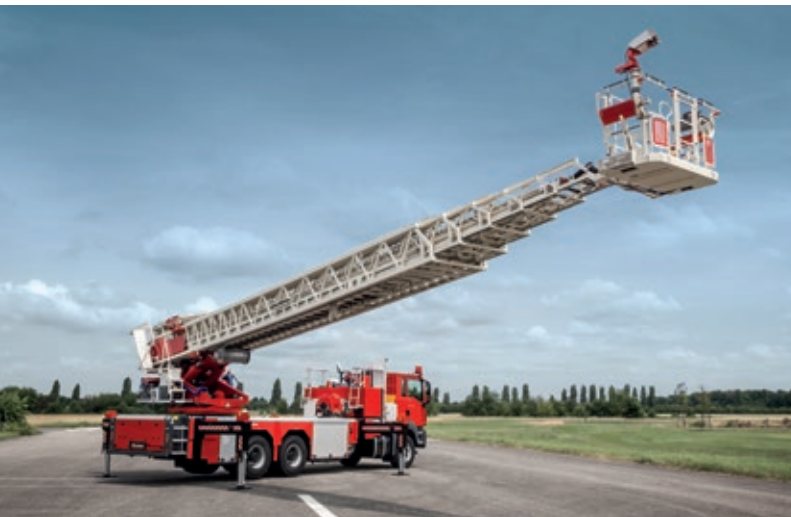
Rosenbauer L64 aerial ladder with normal/high pressure pump, foam proportioning and water/foam tank
