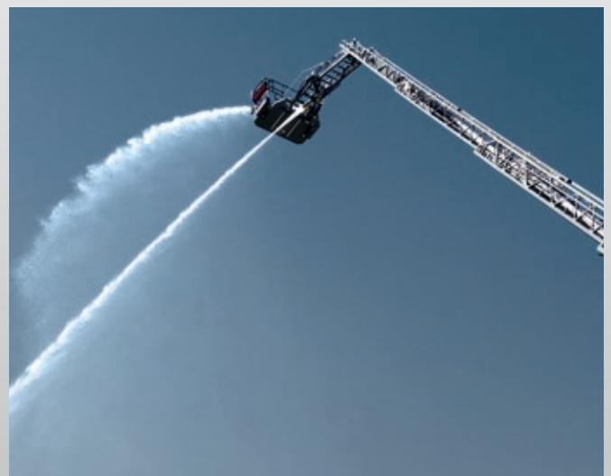
Rosenbauer turntable ladders can be optionally equipped with a large turret directly at the top of the ladder for even greater flow rates.
