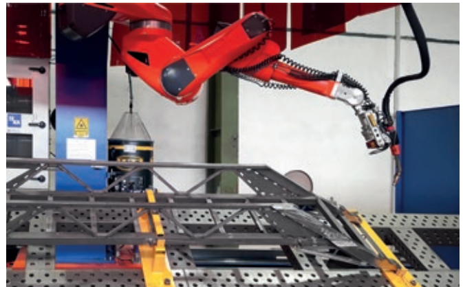
Modern production of the ladder set by means of a robot welding system.
