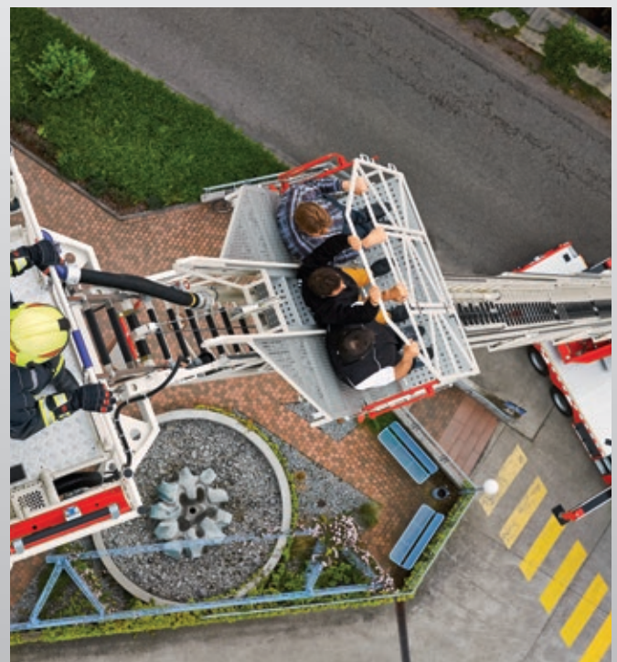
Spacious lift with 270 kg live load
