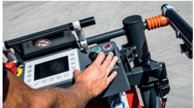
The operation of the turntable ladder is possible regardless of the position of the control panel.
