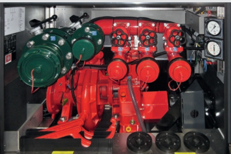
Booster pumps can be installed on any turntable ladder and guarantee a secure supply of water right up to the top of the ladder.
