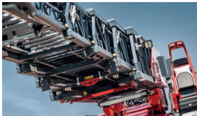
XS ladder set with cut-out for snug fit of the cage boom
