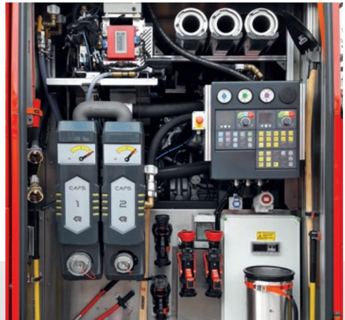
Upon request, Rosenbauer turntable ladders can also be equipped with a CAFS system.
