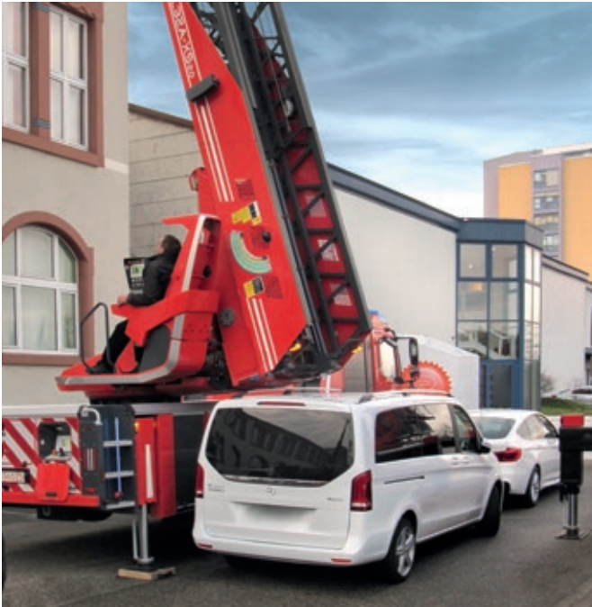
Driving over obstacles is easily made possible by the variable support.
