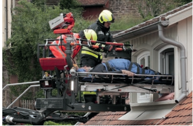
Depending on requirements, the stretcher can be turned either to the left or to the right.
