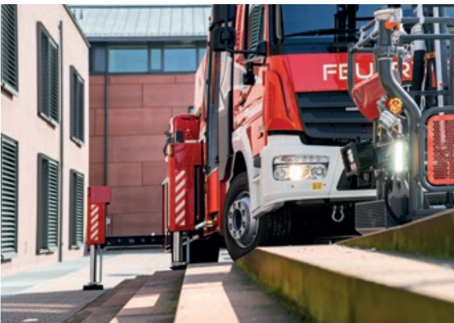
The support width is infinitely adjustable and always permits the maximum reach.
