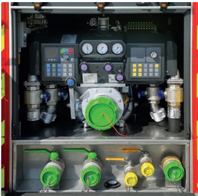
The Rosenbauer NH 45 installed in the rear guarantees optimal utilization of the available space.
