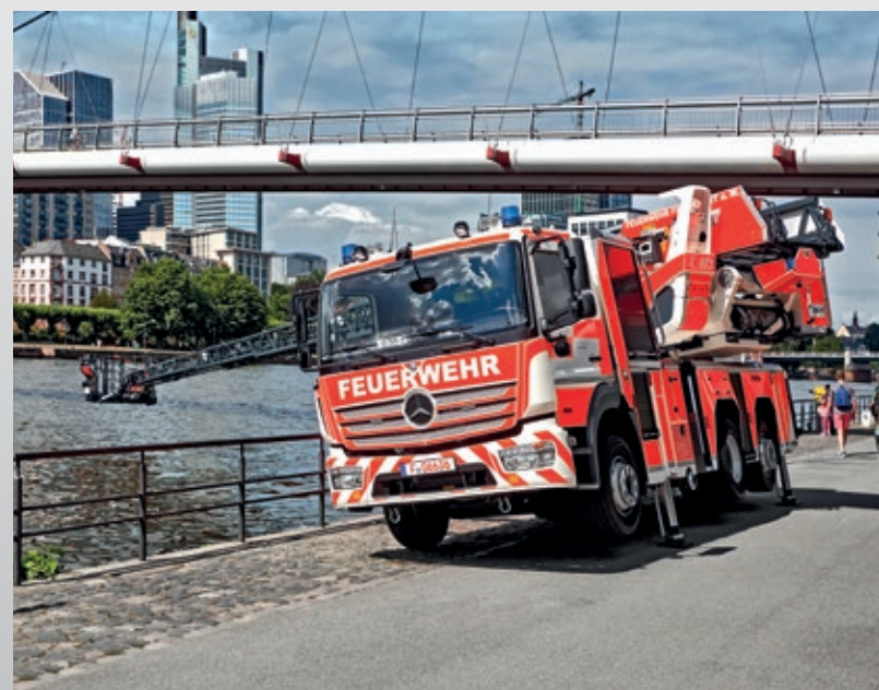
Deliberate inclination of the vehicle to increase the below-ground-level area
