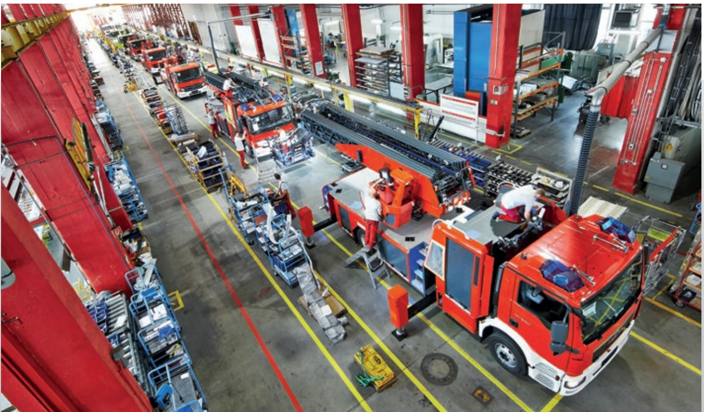
Production takes place within a clocked continuous assembly.
